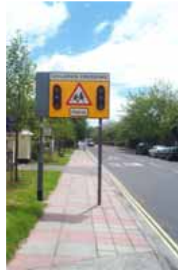
High Visibility SCP Warning Sign with Double Warning Lights – Cockington Primary School (right picture)
