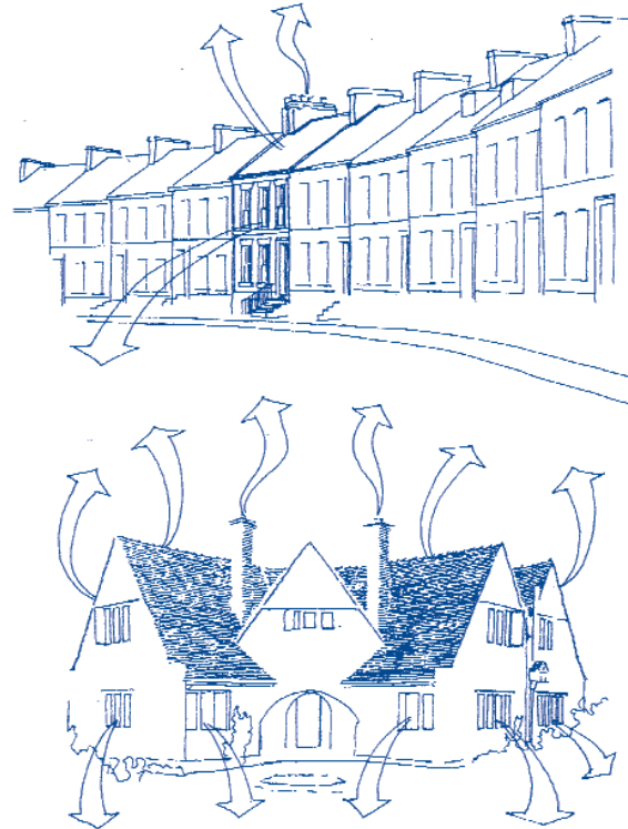
Figure 2: Main points of heat loss from terraced and detached buildings
